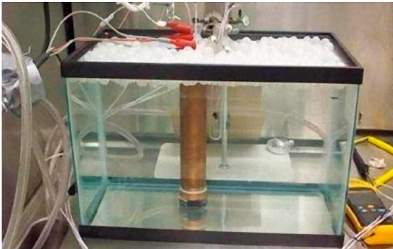
A new “calorimeter,” shown immersed in this water bath, provides the first inexpensive means of identifying the hallmark of cold fusion reactions: the production of excess heat.
